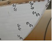
The first step consists in positioning a certain number of coded targets with adhesive tape at strategic positions on the hull; the deck line, the waterline and the bow. Others are positioned to indicate the form of the hull, but in any case, there's no need to place too many on the hull because Rhino reconstructs the surfaces based on definition points by 3D interpolation.
