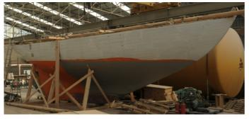
Measuring the hull is the first step in the repair process; a job which is generally tedious and not very precise. However, CNS-Co have been using the Rhinophoto application since the release of the very first version in 2009 and this software has allowed them to carry out the measurement process quickly, easily and precisely.
