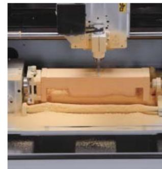
With the optional Rotary Axis Unit, objects can be milled unattended at any angle from 0 to 360 degrees and around multiple surfaces.
