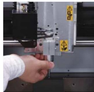
Attach the milling cutter best suited for the material and milling conditions. You can quickly set the origin on screen.
